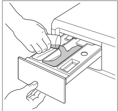
2. If required, pour fabric softener into the compartment marked
